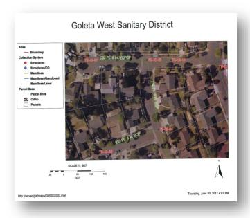
by the field crew and carried in every District vehicle. Each District asset is labeled with a unique identifier. Atlas maps include information such as pipe size, pipe type, manhole depth, pipe segment length and material etc.
