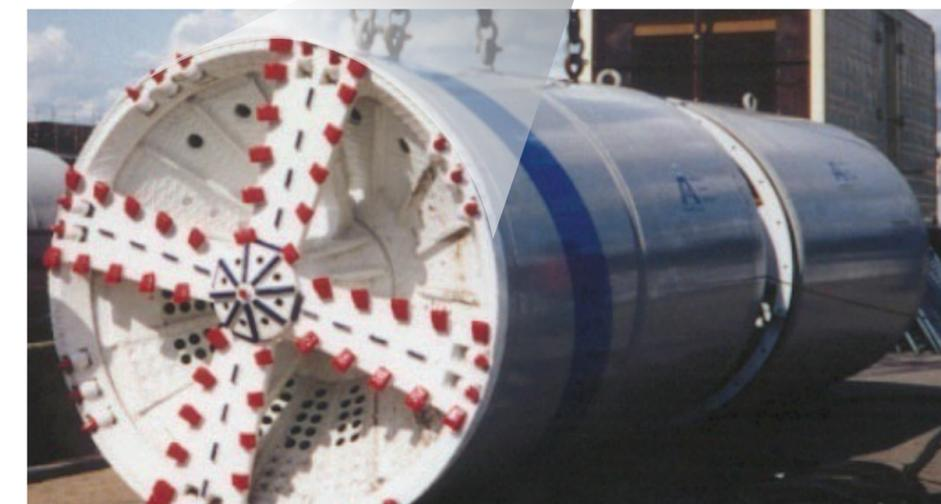
A cutterwheel excavates material at the face of the machine, as shown in Figure 2. A sophisticated laser system ensures that the tunneling operation continues at the correct angle.
