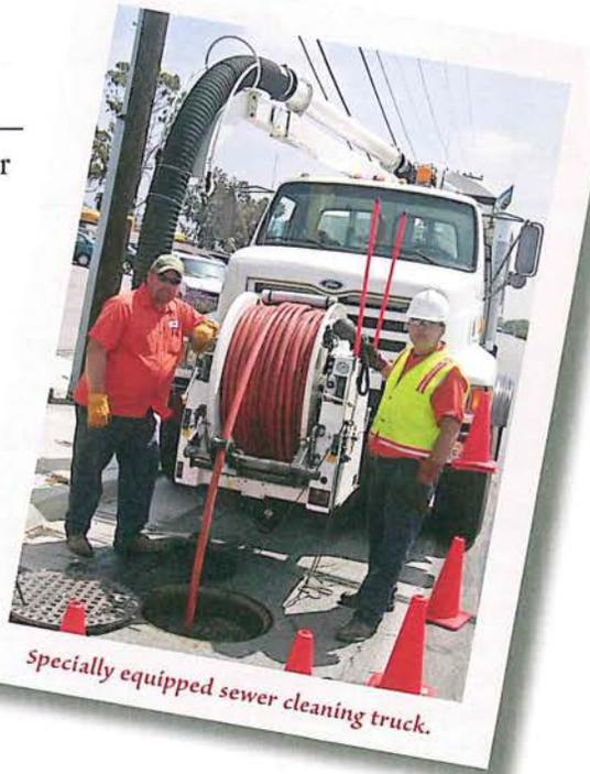
Specially equipped sewer cleaning truck.
