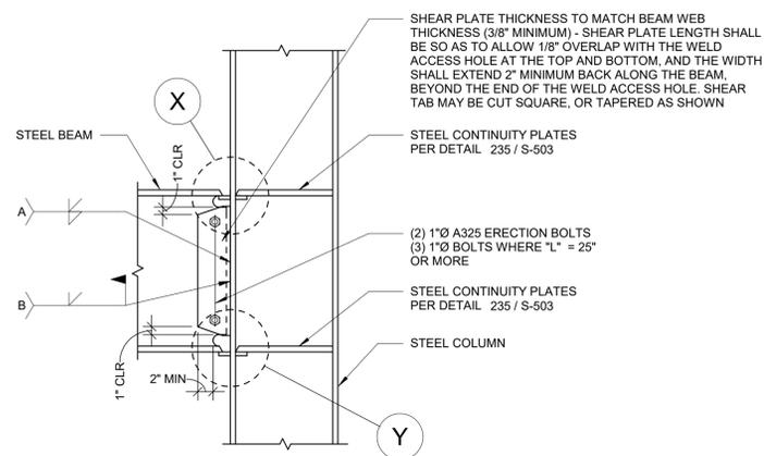
234 TYPICAL SHEAR PLATE AND BEAM FLANGE WELDING AT REDUCED BEAM SECTION (RBS) MOMENT CONNECTION
