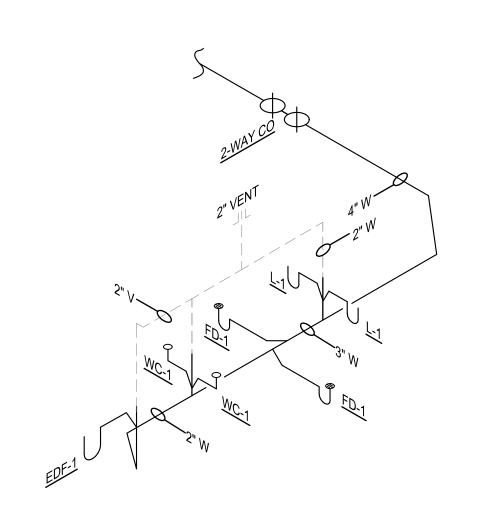
WASTE WATER PIPING SCHEMATIC
