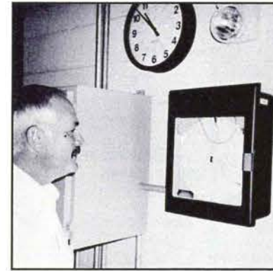
Chief Inspector John Mattingly checks the flow chart to determine the District's average daily flow of wastewater to the treatment plant.
