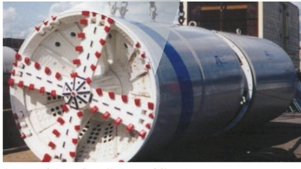
Figure 2. Face of Microtunneling Machine (Courtesy of Akkerman)
